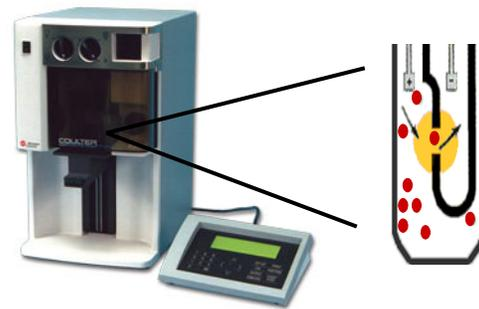
**Figure 3. Z2™ COULTER COUNTER® and aperture.**
